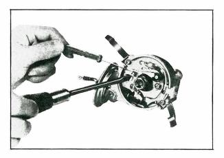
Fig. EE-96 Point Gap Measure
