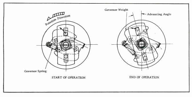
Fig. EE-83 Centrifugal Advance Mechanism
