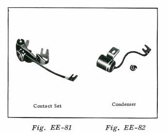
but also increase secondary voltage by switching off quickly primary electric current.
