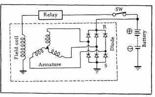
Fig. EE-6 Connection within Alternator
