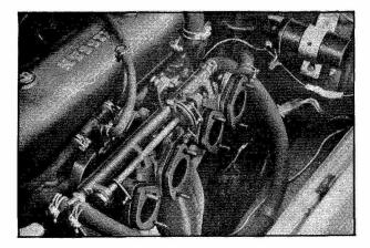
Fig. EM-32 2. Remove Intake manifold to Cylinder head stud nuts.
