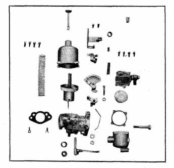
Fig. EF-13 Suction Piston & Suction Chamber
