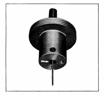
Fig. EF-15 Setting Jet Needle
