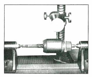
Fig. EE-61 Inspection of Armature Shaft for Bend
