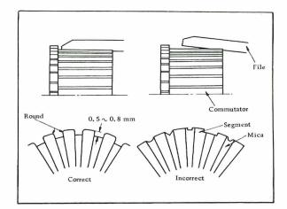
Fig. EE-63 Undercutting Insulating Mica
