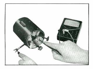
Fig. EE-58 Field Coil Test for Continuity
