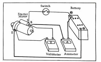
Fig. EE-68 No-load Test
