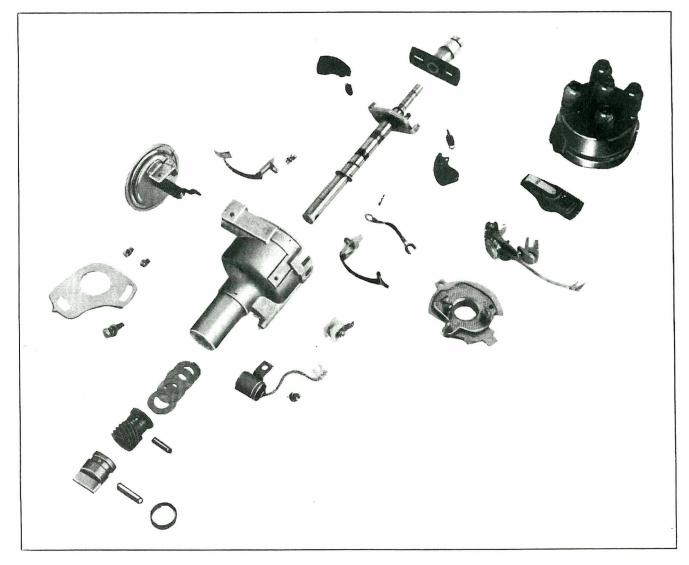
Fig. EE-93 Exploded View of Distributor
