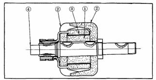
Fig. EE-4 Sectional View of Rotor
