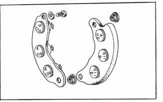
Fig. EE-20 Diode Set Exploded View
