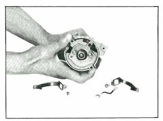
Fig. EE-91 Disassembly of Contact Breaker Plate
