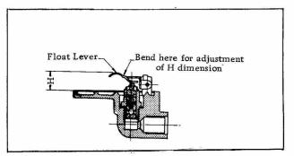
Fig. EF-10 Adjusting Float Level
