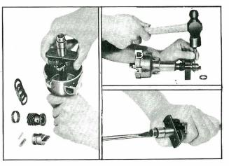
Fig. EE-92 Disassembly of Coupling Shaft and Cam
