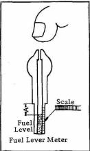
6) If the dimension "A" Fig. EF-28 of the fuel level meter is  $18 \pm 1 \text{ mm} (0.7087 \pm 0.0394 \text{ in.})$ . the fuel level is normal, that is, the fuel level is 20 mm (0.7874 in.) above the center of Main Bore when the fuel pressure is  $0.25 \text{ kg/cm}^2$  (3.55 lb/in<sup>2</sup>).
