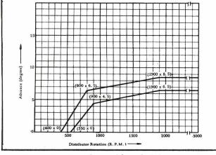
Fig. EE-89 Centrifugal Advance Characteristic
