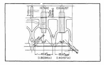
Fig. EM-62 Sectional View of Cylinder Head
