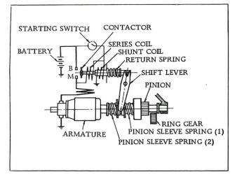
Fig. EE-52 Starting Motor Circuit
