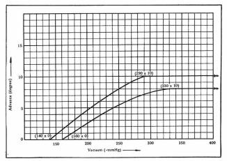
Fig. EE-87 Vacuum Advance Characteristic
