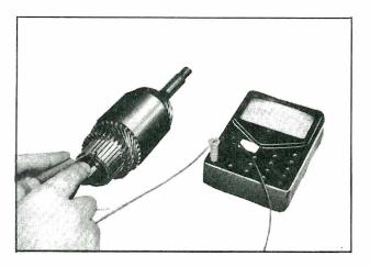
Fig. EE-66 Armature Test for Continuity
