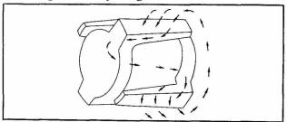
Fig. EE-5 Magnetic Circuit
