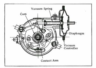
Fig. EE-84 Vacuum Advance Mechanism
