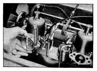
Fig. EF-16 Carburetor Balancing
