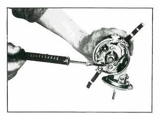
Fig. EE-95 Point Pressure Test
