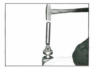
Fig. EE-56 Removal of Over-running Clutch Ass'y
