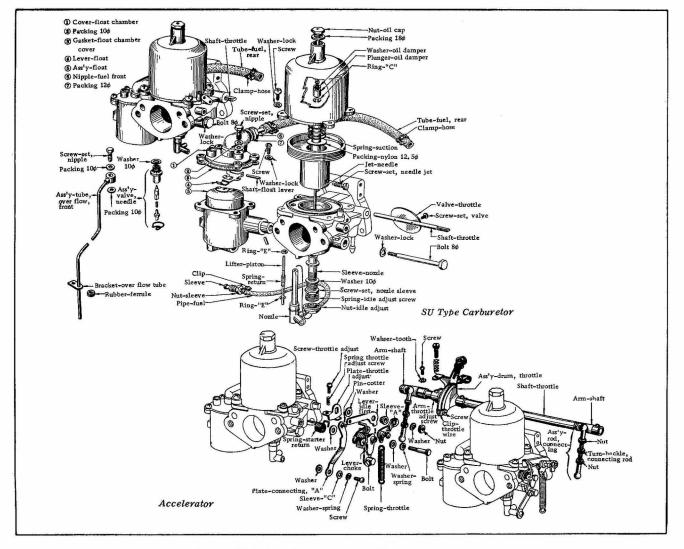
Fig. EF-17 Carburetor Component Parts
