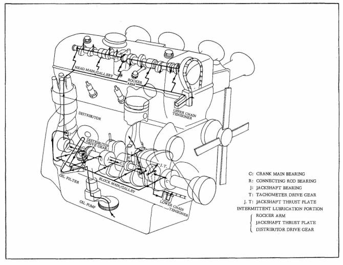
Fig. EL-1 Lubrication Circuit
