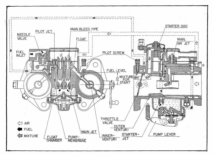
Fig. EF-19 44PHH Fuel Flow Chart
