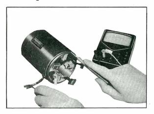
Fig. EE-59 Field Coil Tester Ground
