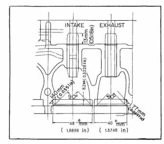
Fig. EM-58 Sectional View of Cylinder Head
