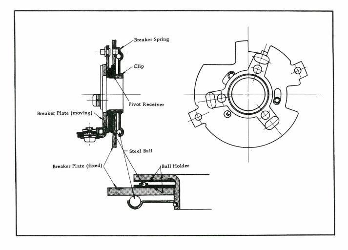
Fig. EE-88 Breaker Plate Collecting Part Mechanism
