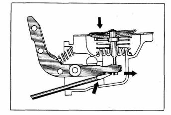
Fig. EF-5 Pull Rod Removal
