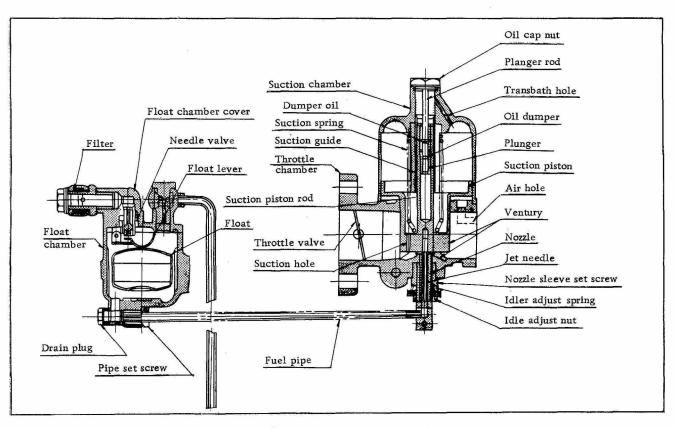
Fig. EF-7 Sectional View of Carburetor
