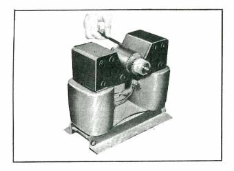
Fig. EE-65 Armature Test for Short
