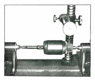
Fig. EE-62 Inspection of Commutator
