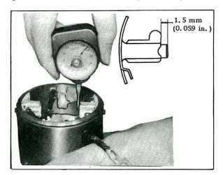
Fig. EE-60 Inspection of Brush Spring Tension
