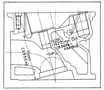
Fig. EM-57 Sectional View of Cylinder Head
