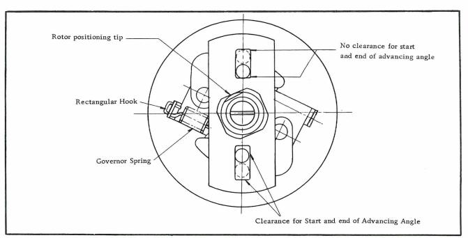
Fig. EE-94 Setting of Governor Spring and Cam
