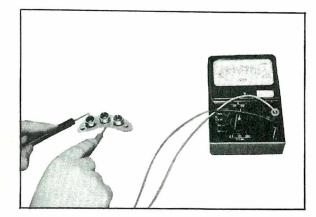
Fig. EE-35 Negative Diode
