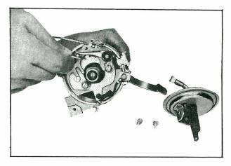
Fig. EE-90 Disassembly of Vacuum Controller
